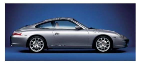
▲ 18-inch GT3 wheels The 18-inch GT3 alloy wheel uses a tough yet lightweight 'flowformed' construction to achieve a further reduction in unsprung weight. The open-spoke design helps to maximise brake performance by enhancing heat dispersal.
